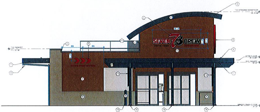
1 EXTERIOR ELEVATION - LEFT SIDE 3/8" = 1'-0"
